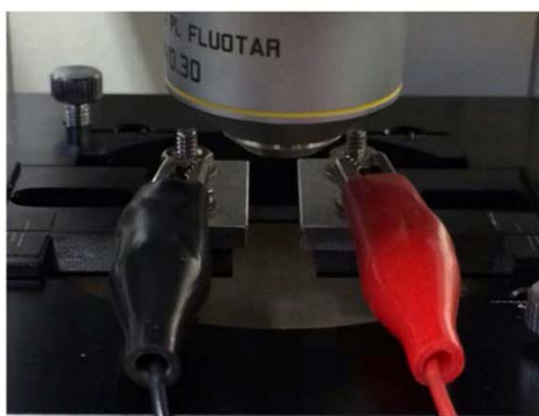
Figure 9. (a) Strain sensitivity of a sample conductivity during imaging and (b) the experimental setup, with a test sample loaded onto the tensile testing stage. [Color figure can be viewed in the online issue, which is available at wileyonlinelibrary.com .]
